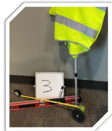
An example of some of the tools used to conduct a sidewalk inventory, including a high-visibility safety vest, a measuring wheel, a tape measurer, a digital level, and a dry erase board.
