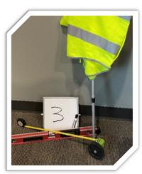
An example of some of the tools used to conduct a sidewalk inventory, including a high-visibility safety vest, a measuring wheel, a tape measurer, a digital level, and a dry erase board.
